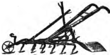
FIG. 25.—This form of one-horse cultivator is well suited for garden work. It can be adjusted in width to suit all rows.
